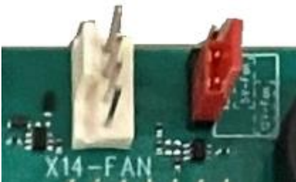
Figure 13: Fan Connector with 4 pins (X14) and Fan Jumper (X38)
