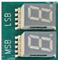
Figure 42: Port 80 BIOS Debug Code 7-Segment Display
