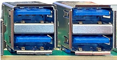
Figure 7: USB 3.2 Double Connector (X32, X33)
