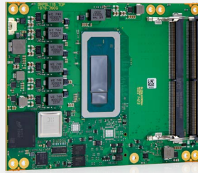
COM Express® basic form factor JUMPtec® COMe-bRP6 (E2) (pin-out Type 6 compliant)
