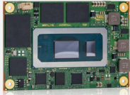
COM Express® mini form factor JUMPtec® COMe-mRP6 (E2) (pin-out Type 10 compliant)
